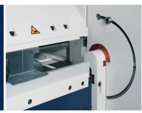
Usage of sharp-nose or segmented tools up to 90 mm by manual height adjustment of the clamping beam. The bending angle will be adjusted on the
