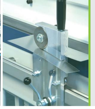
The cutting device is used for safe and easy cutting of ST37 sheets with a material strength of up to 0.8 mm.
