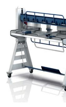
Rear view: 2 variable gauge arms with scale movable on linear guide incl. 2 tipping gauges
