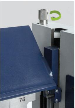
Clamping beam force adjustment
