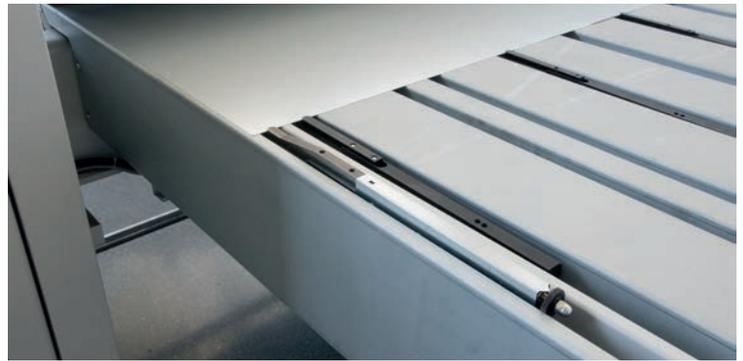
Picture above: Standard back gauge with retractable support plates.
