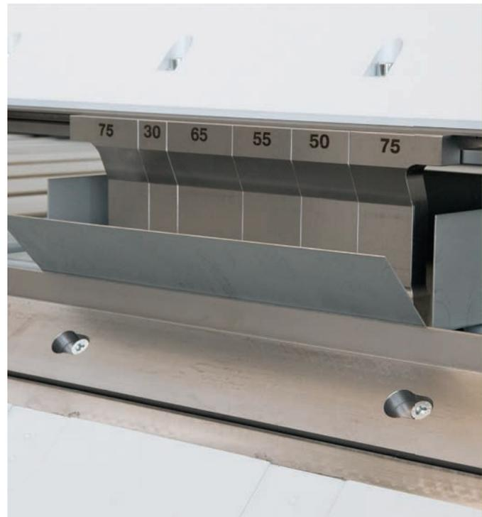
Bending up to 110 mm high boxes with the MAKU is simple and easy.
