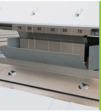
Crowning device for folding beam: manual central crowning device (not in combination with cranked folding blades)
