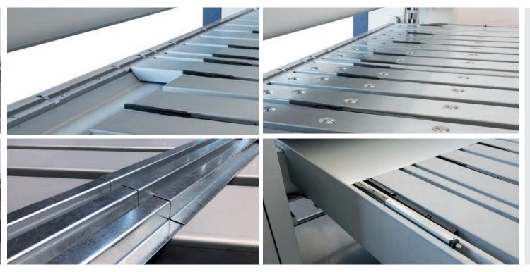
Picture above: Standard back gauge with retractable support plates. Picture below: Thanks to the new option for conical bending profiles can be connected to each other very easily.
