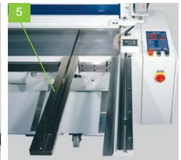
Movable sheet support with T-slots on linear guide
