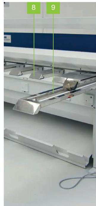
Table with exchangeable stainless steel plates with recessed grips [8] and extended angle gauge on the right with scale incl. lateral flip gauge on linear guide [9]
