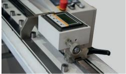
Optional for PDC and PDC-NC: Extended angle gauge (right or left) with electronic length measurement system incl. lateral flip gauge on linear guide
