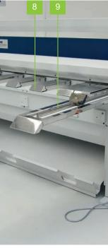
Table with exchangeable stainless steel plates with recessed grips [8] and extended angle gauge on the right with scale incl. lateral flip gauge on linear guide [9]
