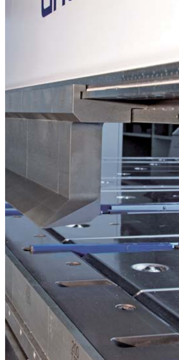
Segmented goat's foot blade, hydraulic tool clamping.
