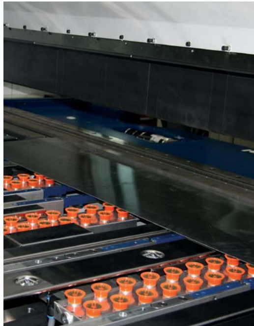
With the suction gauge all bends on one side can be handled with one simple move by the operator.
