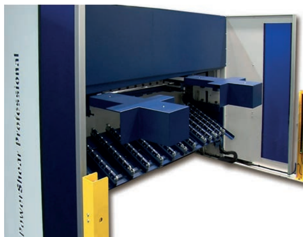
Rear view: Motorized back gauge and sheet support as well as rear light barrier
