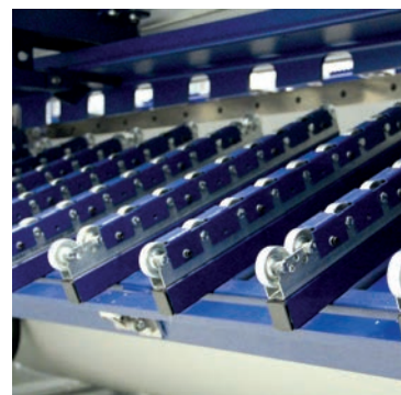
Sheet support, pneumatically controlled
