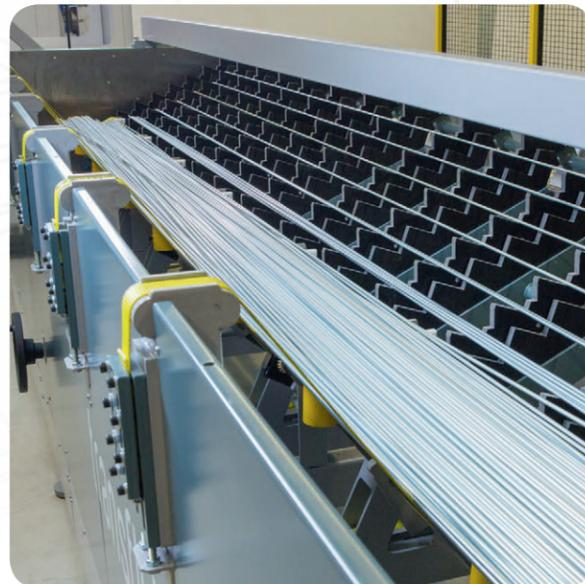
Step belt conveyors, also optimally suitable for small, long tubes
